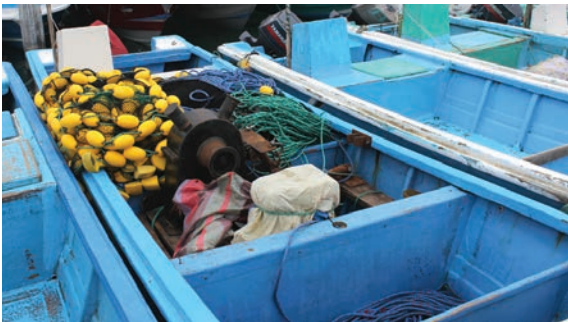
Figure 6. Open boat with purse seine gear at Anconcito, Ecuador. See the small winch on the center of the boat. Photo: F. Félix.
