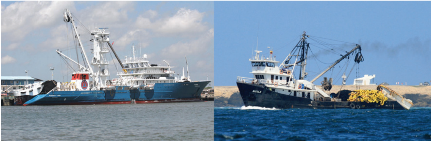
Figure 2. Ecuadorian industrial purse seiners. Left: tuna vessel; right: small pelagic vessel. Photos: F. Félix.
