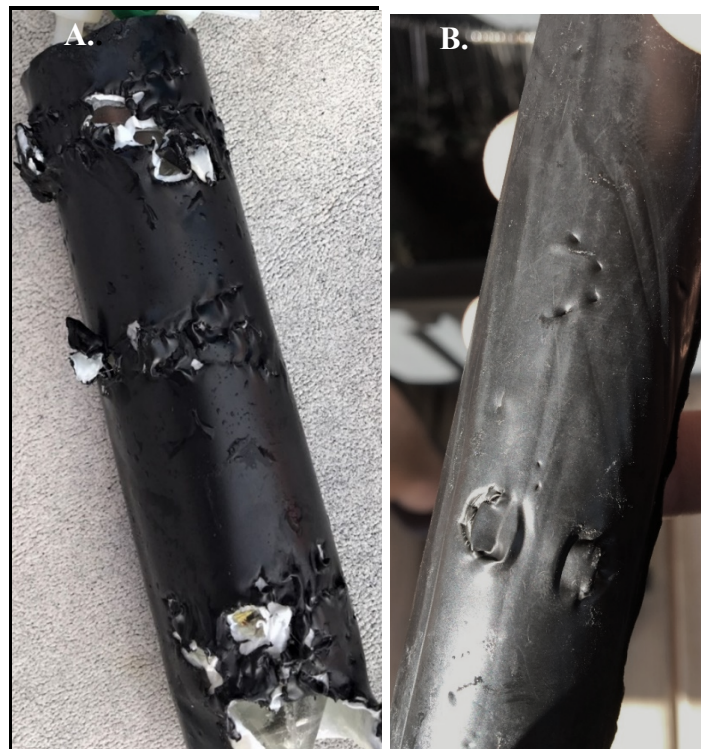
Figure 4. Visual inspection of devices showed (a.) shark bite marks and of (b.) bite marks other fish species.
