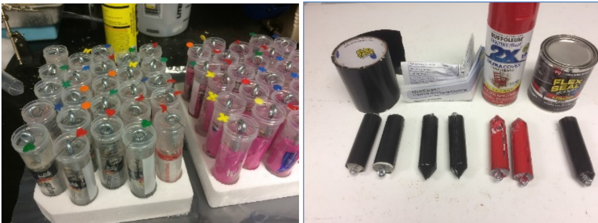
Figure 1. Decoys drying in in their molds (left) and later covered using various coatings (right). The final decoy coating used was Flex Tape ® (far left of the photograph on the right).
