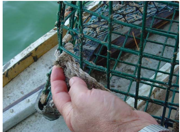
2006 Barium Sulfate Groundline Batch 1 fished by Elliott Thomas; Signs of Chaffing at trap end of bridle
