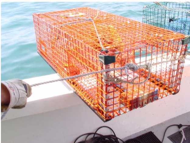
2005 Barium Sulfate Sinking Line fished by Pat White shows no sign of wear in year 2 fished on gravel bottom.
