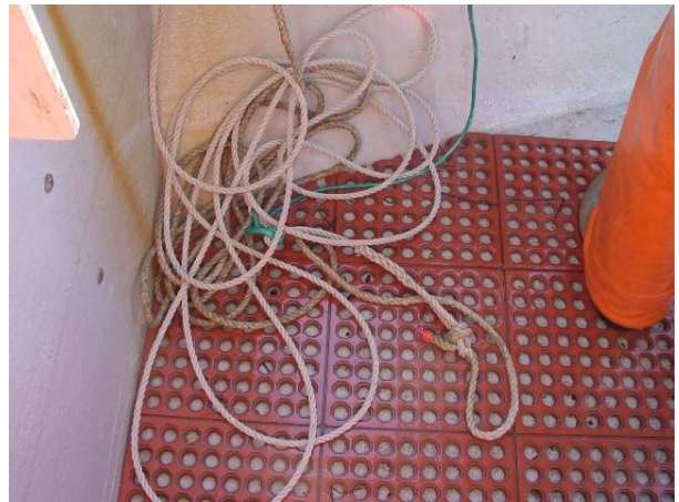
2006 Barium Sulfate Groundline Batch 1 as it is hauled on deck
