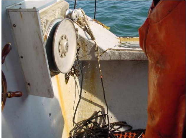
2006 Stiff endline made of 3/8" outer diameter rubber as it is hauled by Elliott Thomas.
