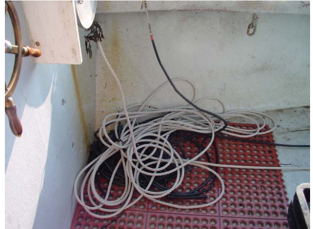
2006 Stiff endline made of 3/8" outer diameter rubber as it coils on deck while being hauled by Elliott Thomas.
