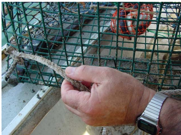
2006 Barium Sulfate Groundline Batch 1 fished by Elliott Thomas; Signs of Chaffing at trap end of bridle
