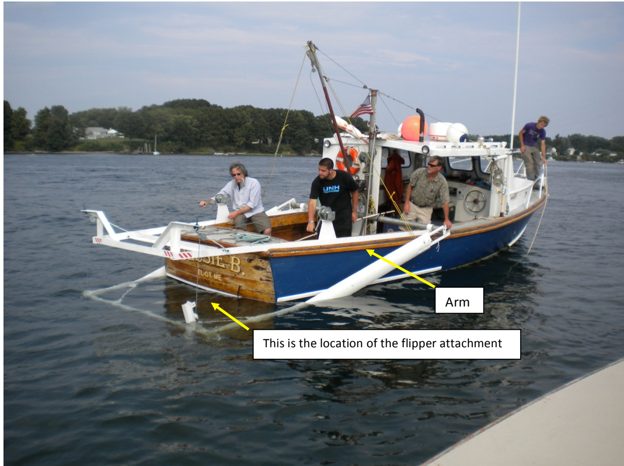
Figure 2-3. The flipper deployment frame mounted on the Jesse B . The flipper is lowered to a position under the vessel when the 'arms' are in a vertical position
