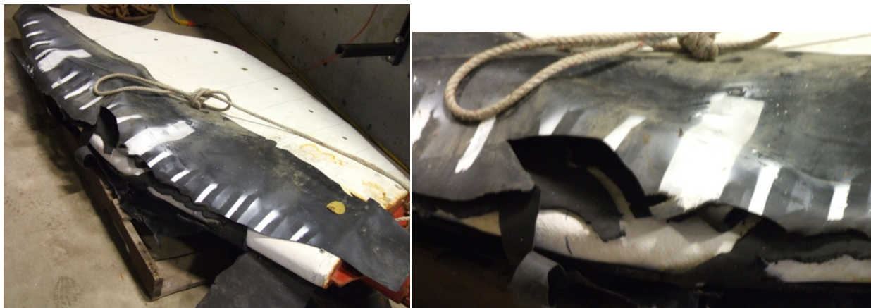
Figure 2-7. A series of after the fact pictures showing the status of the leading edge of the flipper. The top two pictures show a scalloped edge which is most likely resulting from a 'sawing action' of the line as the float descended.
