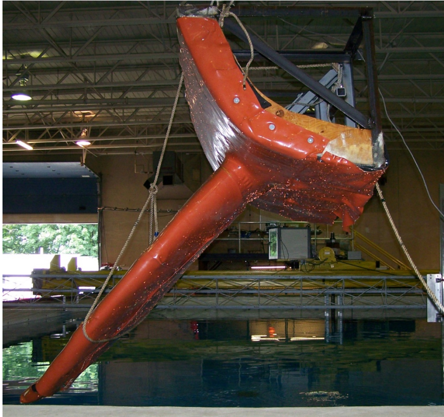
Figure 2-1. Completed flipper-whale body section while being weighed in air and water at UNH Chase Ocean Engineering Lab.
