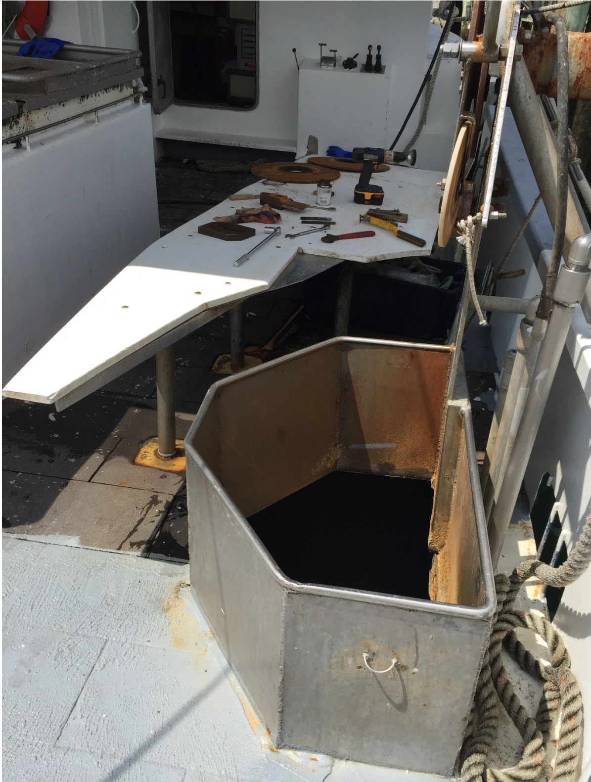
Figure 1.5: Rope locker and pot hauler. This rope locker is about 4' x 6' x 6' and can hold the line for three complete trawls of 50 traps each. During hauling, sometimes a crew member is stationed in the rope locker to ensure that the line coming into the locker is coiled neatly.
