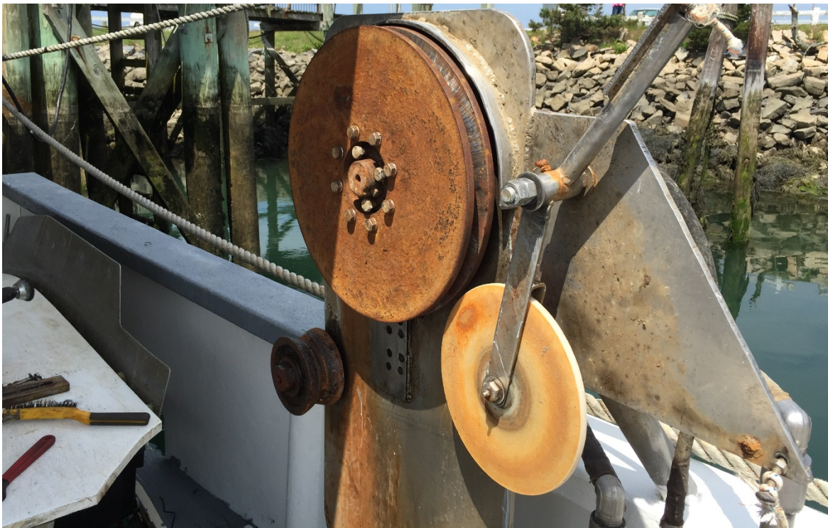
Figure 1.3: Pot Hauler with plates adjusted for 5/8" rope.
