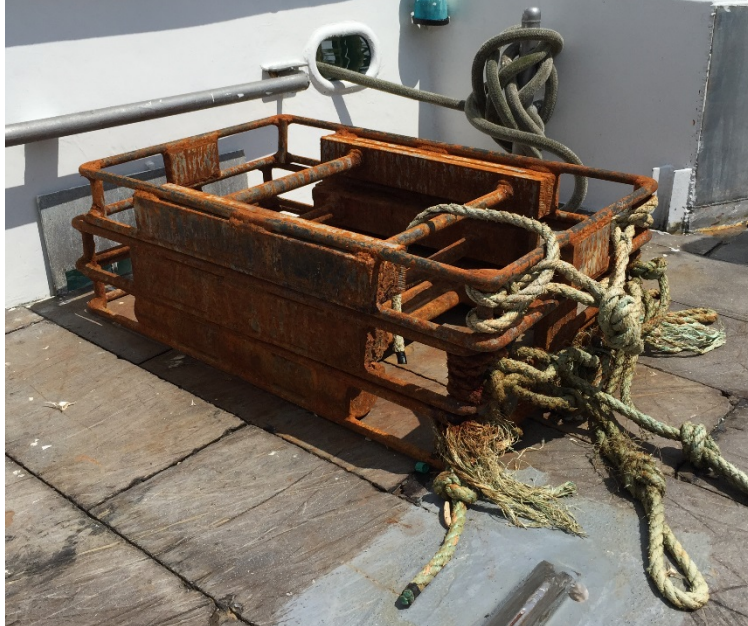
Figure 1.2: Two 180-pound steel anchor sleds. The anchor sleds weigh more than the empty line pack spool (about 135 pounds), i.e. the line pack spool weight is comparable to weights of existing gear.
