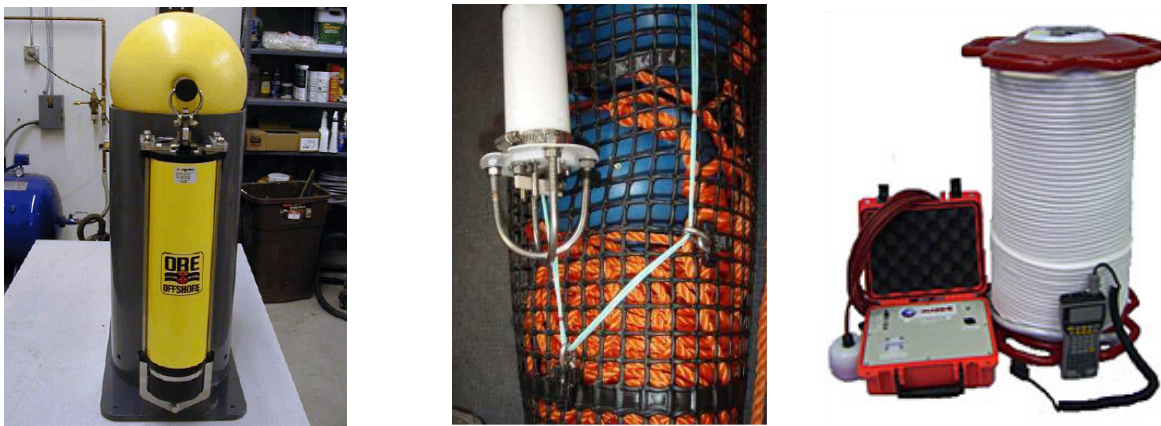
Figure 2.2: Three line pack methods. Left: Line canister (ORE Offshore). Middle: Mesh bag as line canister (Liggins and Westley, 2011). Right: Line Spool (FioBuoy, FioMarine).
