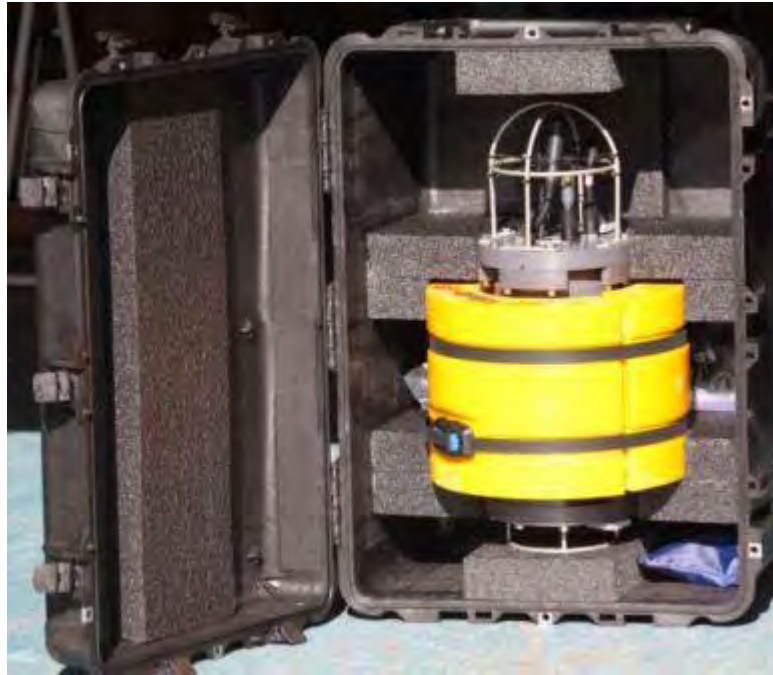
Figure 4: JASCO's Autonomous Multi-channel Acoustic Recorder (AMAR).
