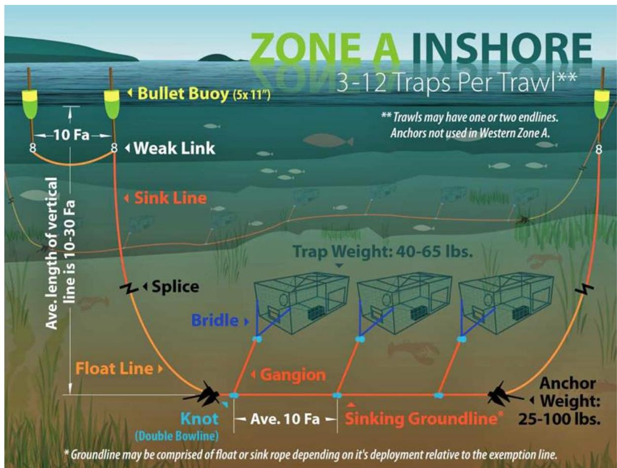
**Figure 25.** An illustration of a lobster gear configuration in the Gulf of Maine (Zone A Fishing Zone). There may be more than one endline (buoy line) on a lobster trawl, typically when the number of pots reaches five or more, but sometimes fewer. Fa = fathoms. (Illustration from McCarron and Tetreault, 2012).
