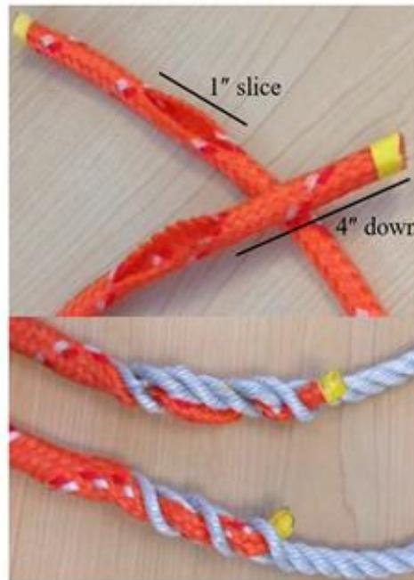
**Figure 8.** *Novabraid* sleeve assembly diagram
