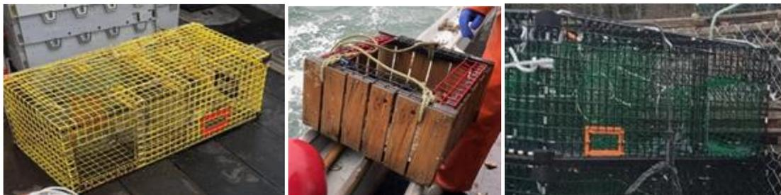
**Figure 10.** Lobster (left), whelk (center) and black sea bass (right) traps used during field testing.
