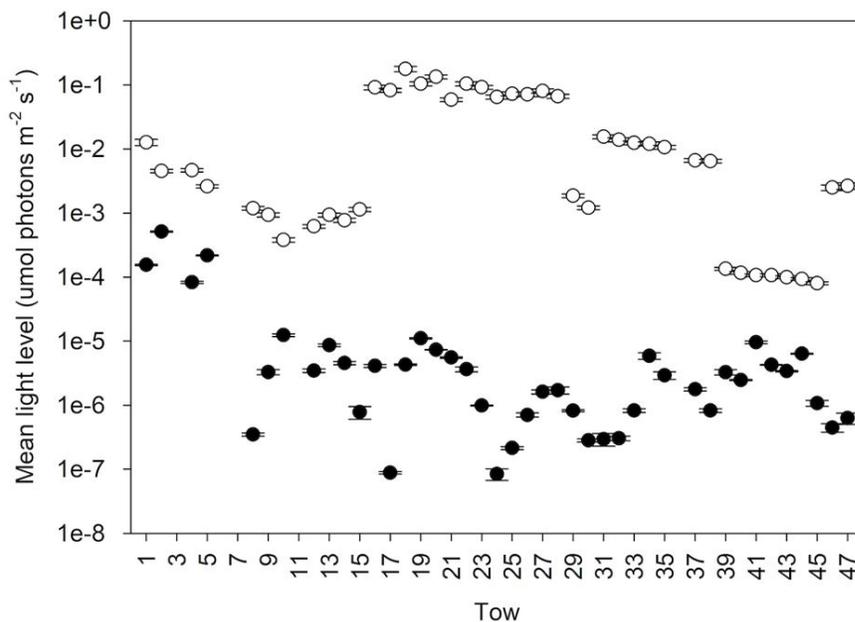
Figure 3. Mean light level measured at the center of the fishing line for the unilluminated trawl (closed circles) and illuminated trawl (open circles) per tow.  $\pm$  bars are standard errors ( $n = 50$  measurements per net per tow).
